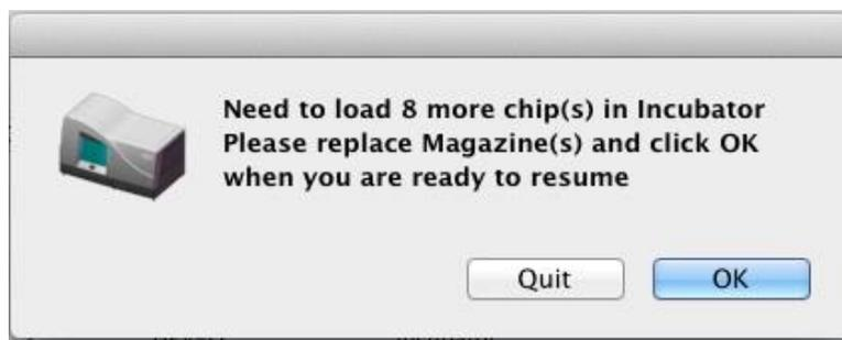
When the OK button is clicked, the system checks the magazine resources. The same message will be prompted again if the correct number of microarray chips are not found. The operator can reload the magazine again or click “Quit” to abort the run.
