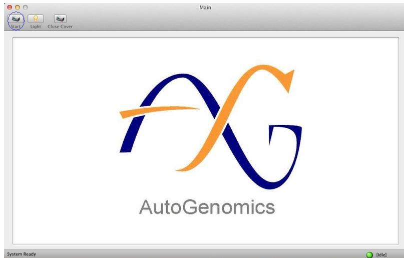
The light button (located next to the Start button).can be clicked to turn on or off the light. The light will stay on for approximately 15 minutes before it will automatically turn off. This light will also automatically turn off when the cover closes.
